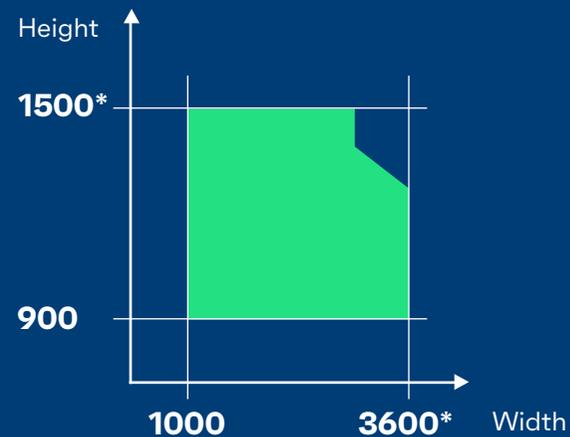
\*Max dimensions and weights depend on multiple parameters including wind load requirements and glass type choice.
